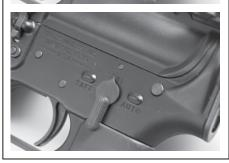
When the magazine is emptied, the bolt will lock open. In order to fire, you need to press the bolt catch to release the bolt.
